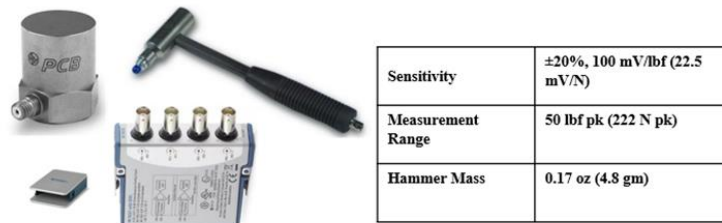
Fig 6: Apparatus used for experimental testing: [clockwise from top left] accelerometer, impact hammer, data acquisition card.
