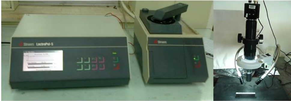
Fig. 2 Optical microscope and electro polish machine used
