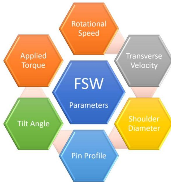
**Fig 2: Main parameters of the FSW process**
