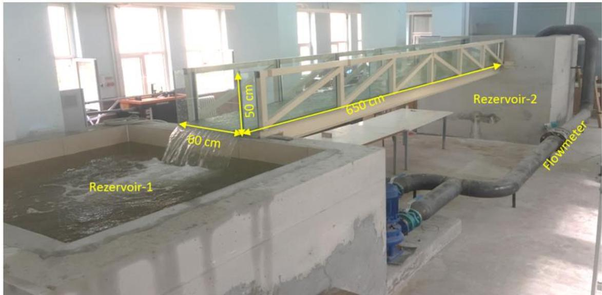
Fig 4: Open channel system used in experiments.
