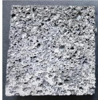
**Fig. 2 Aluminum foam sample produced**
