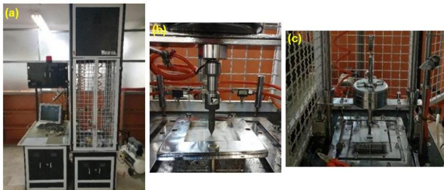
Fig. 4 Drop weight device (a) General scheme (b) Moment of impact on the specimen (c) pneumatic jack equipment for secondary impact prevention
