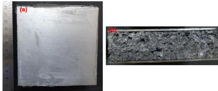
Fig. 3 Sample Sandwich Composite Plate with Aluminum Case (a) Front View (b) Side View
