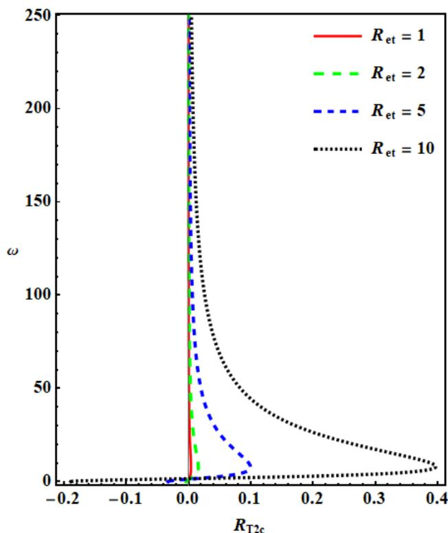
**Fig. 1:** Plot of  $R_{T2c}$  versus  $\omega$  for different values of  $R_{et}$  with  $P_{rD} = 2$ ,  $\eta = 0.2$  and  $\varepsilon = 0.5$ .
