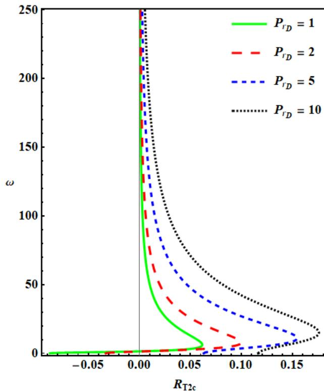
**Fig. 4:** Plot of  $R_{T2c}$  vs  $\omega$  for different values of  $P_{rD}$  with  $\varepsilon = 0.5$ ,  $R_{et} = 5$  and  $\eta = 0.2$ .
