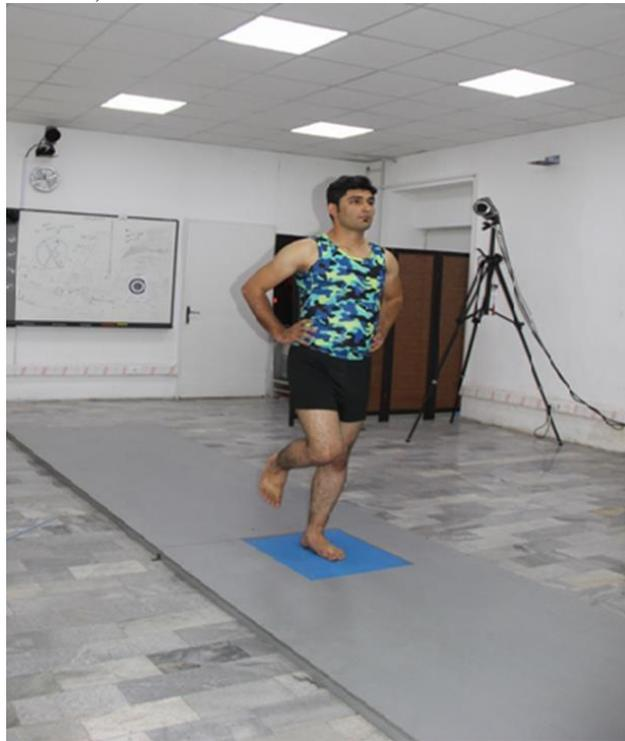
Figure 1: test position while doing tests on a force platform (experimental setup)
