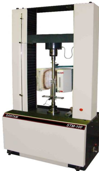
Figure 5: Creep apparatus used in the present study
