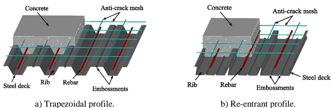
**Figure 1.** Typical layout of composite slabs.
