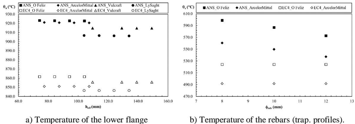
**Figure 6.** Comparison between the numerical results and EN 1994-1-2 provisions for the fire resistance class R60.
