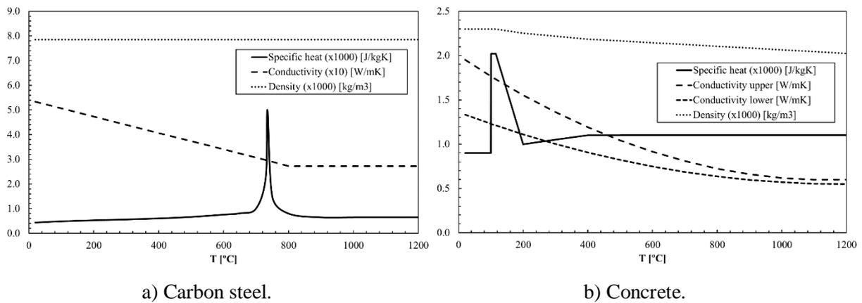
**Figure 3.** Thermal material properties.
