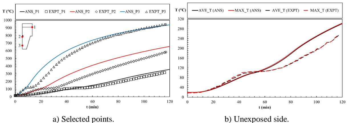
**Figure 5.** Numerical and experimental results – Points 1, 2 and 3 at distance 20, 74 and 123 mm from the top.
