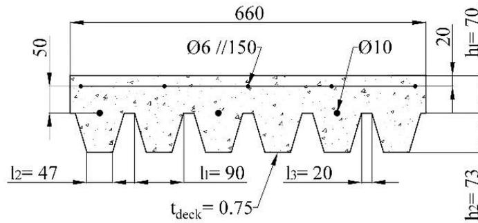
**Figure 4.** Cross section of the tested slab: dimensions in millimetres [2].
