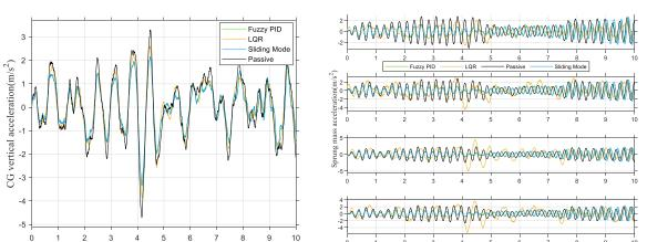
the vehicle mass center (bounce acceleration) and the sprung mass acceleration of each corner of the vehicle.
