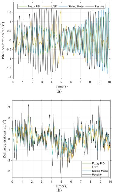
(b) **Figure 7.** Angular accelerations during the test via SAVGS model (a) Pitch angular acceleration (b) Roll angular acceleration
