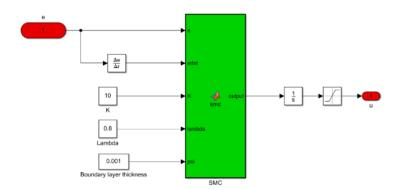
Figure 6. Simulink diagram from the sliding mode controller
