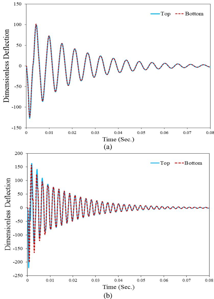
**Figure 5.** Dimensionless displacement of a sandwich plate ( $a/h = 10$ ) with a viscoelastic core with a ratio of ( $E_{\infty}/E_{eq} = 0.5$ ) and relaxation time ( $\tau=0.0001$ ): a) thin sandwich plate ( $a/h=10$ ), b) thick sandwich plate ( $a/h=4$ )
