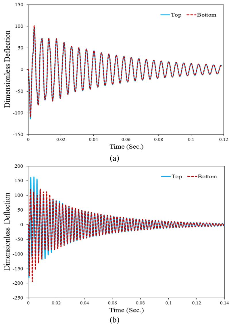
**Figure 6.** Dimensionless displacement of a sandwich plate with a viscoelastic core with a ratio of ( $E_{\infty}/E_{eq} = 0.8$ ) and relaxation time ( $\tau=0.0001$ ): a) thin sandwich plate, b) thick sandwich plate.
