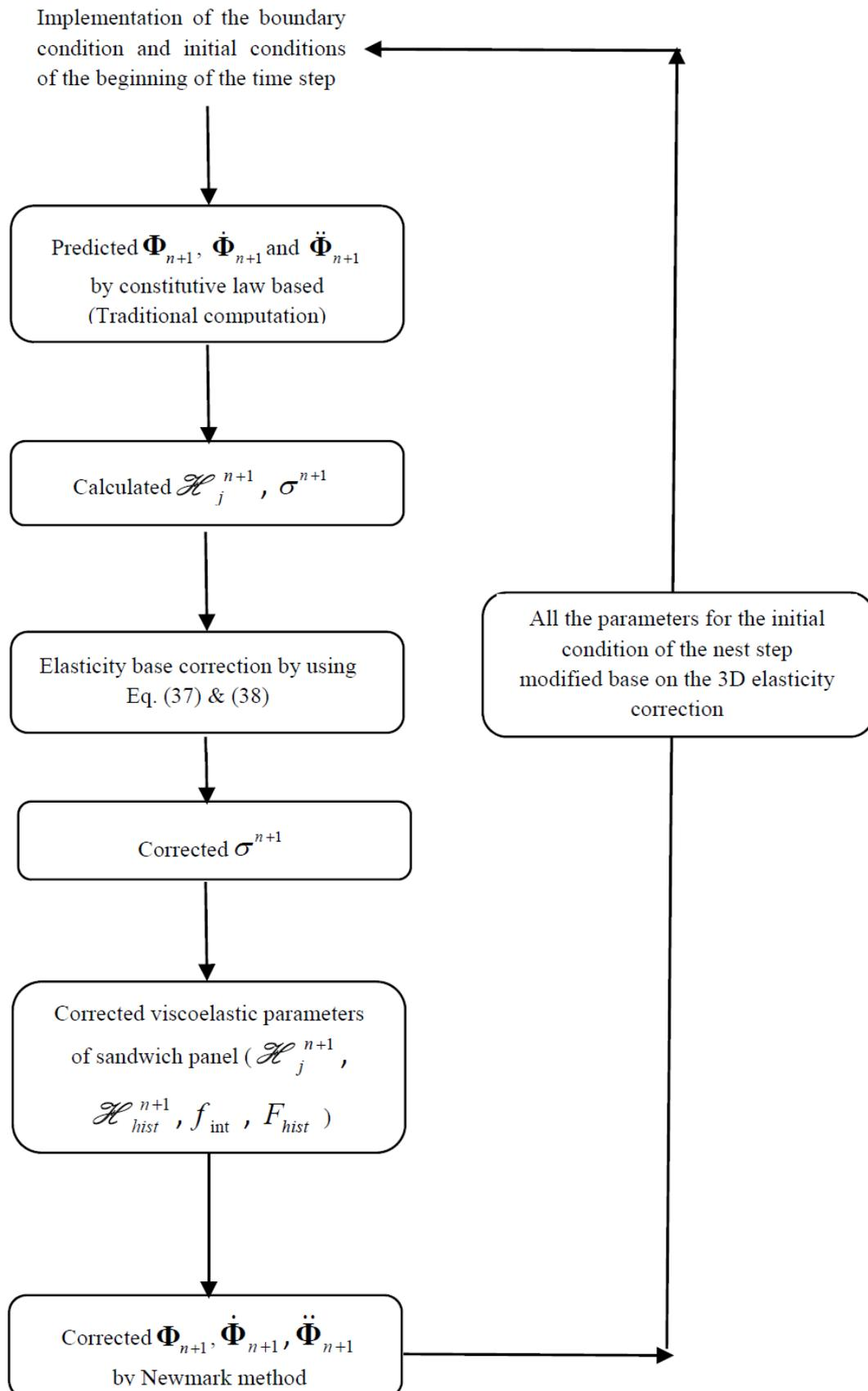
**Figure 1.** Details of the proposed algorithm for correction of all components of the present displacement-based solution.
