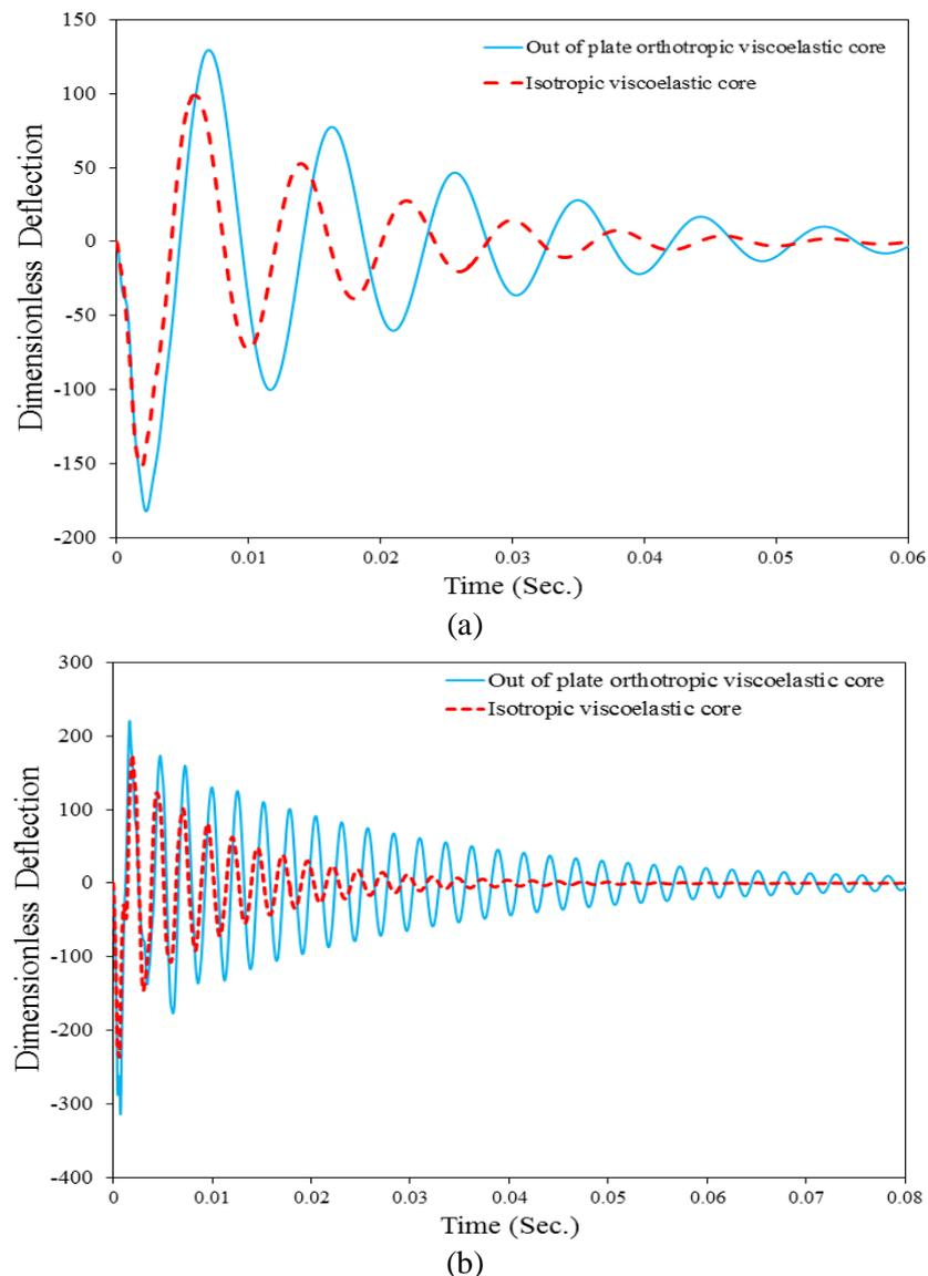
**Figure 10.** The effect of the transversal orthotropic nature of the viscoelastic core compared to the isotropic viscoelastic core on the dimensionless transverse displacement of the middle point of the plate: a) thin sandwich plate ( $a/h = 10$ ); b) thick sandwich plate ( $a/h = 4$ )
