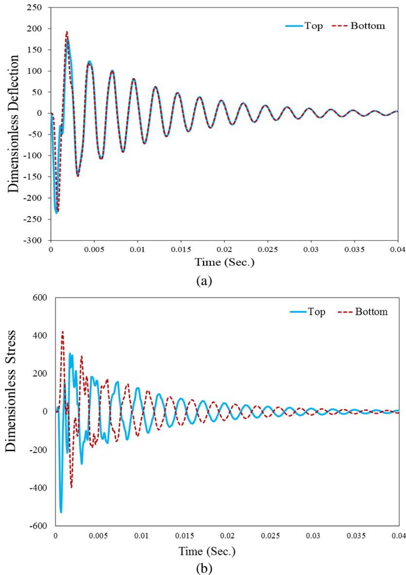
**Figure 4.** Thick sandwich plate ( $a/h = 4$ ) with a viscoelastic core with a ratio of  $(E_\infty/E_{eq} = 0.2)$  and relaxation time of  $\tau = (\eta/E) = 0.0001$  : a) dimensionless displacement, b) dimensionless stress
