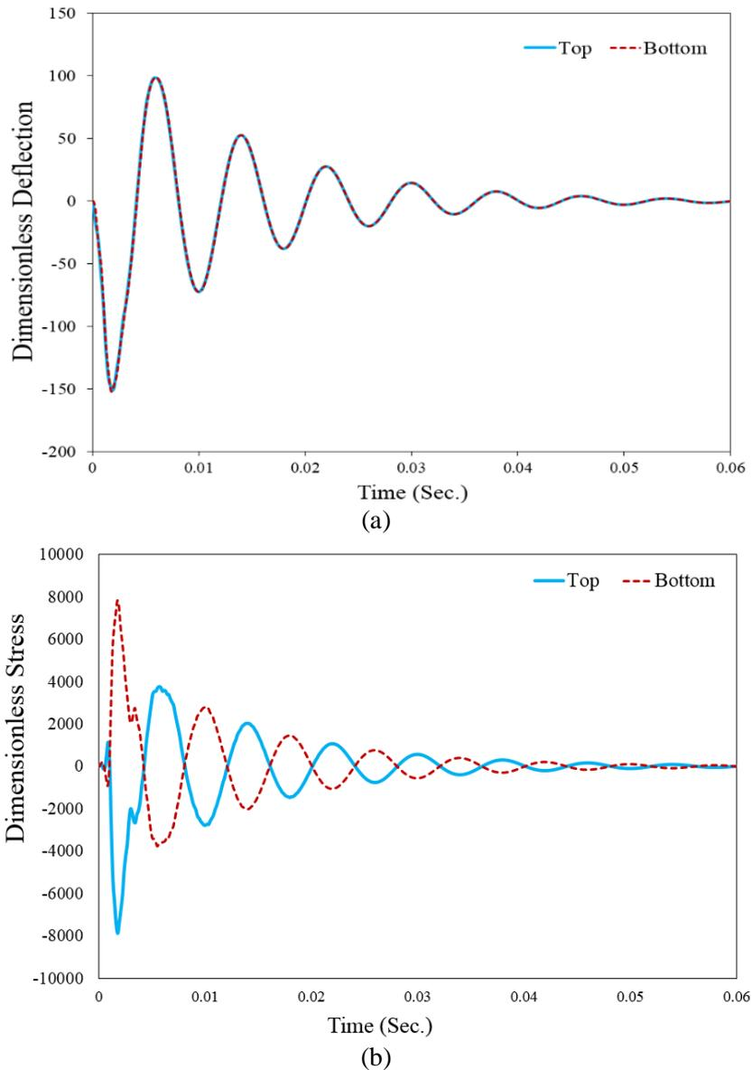
**Figure 3.** Thin sandwich plate ( $a/h = 10$ ) with a viscoelastic core with a ratio of ( $E_{\infty}/E_{eq} = 0.2$ ) and relaxation time of  $\tau = (\eta/E = 0.0001)$  : a) dimensionless displacement, b) dimensionless stress.
