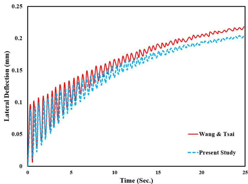
**Figure 2.** A comparison between time histories of lateral deflection of the central point of an isotropic and homogeneous viscoelastic plate by present approach and Wang and Tsai [48] under a step loading.
