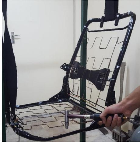
**Figure 4.** Performing the modal testing on the car seat frame
