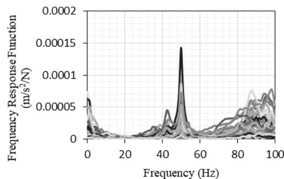
**Figure 5.** The frequency response function of the car seat frame obtained from modal testing
