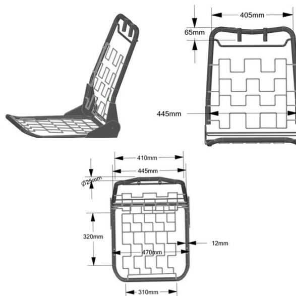
**Figure 1.** The geometric model of the car seat frame with dimensions
