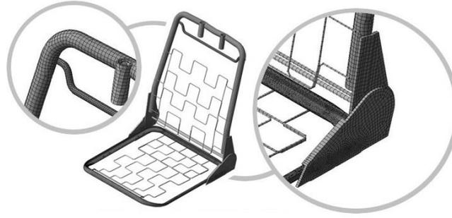
**Figure 2.** The discretized FE model of the car seat frame
