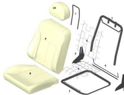
**Figure 3.** The exploded view of the car seat model: 1. Back Frame, 2. Base Frame, 3. Recliners 4. Recliner Mechanism's Rods, 5. Base Suspension Springs, 6. Back Suspension Springs, 7. Headrest Rods 8. Base Cushion, 9. Back Cushion, 10. Headrest Cushion
