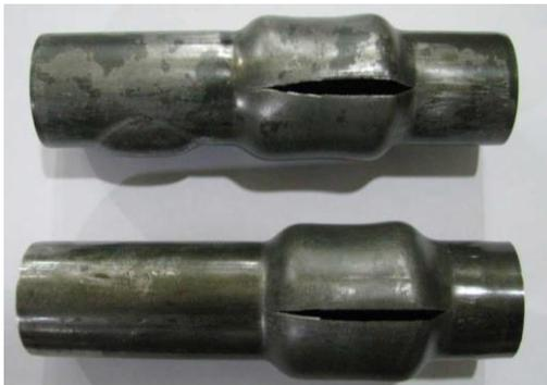
Figure 17. tearing in weld seams in stainless steel tubes.
