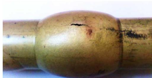
Figure 22. bulge test undertaken on the 70/30 brass tube and tearing occurred in thickness about 0.73mm.
