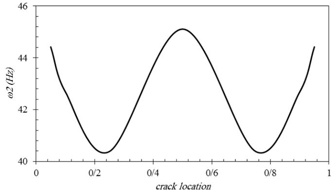
Figure 13. variations of second frequency of plate against crack location ( $h/a = 0/1$ )
