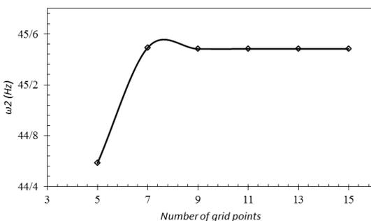
Figure 7. variations of second frequency of plate against the number of nodes
