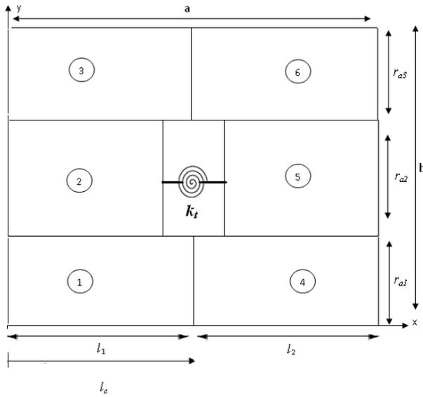
Figure 2. Cracked plate modeling
