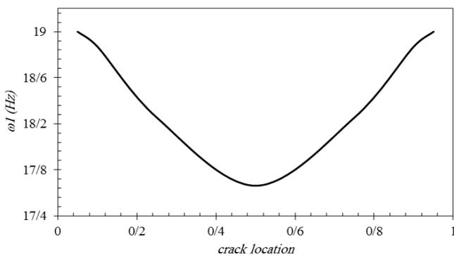
Figure 12. variations of first frequency of plate against crack location ( $h/a = 0/1$ )
