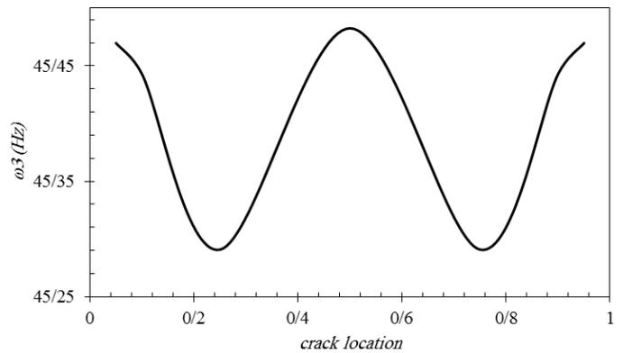
Figure 14. variations of third frequency of plate against crack location ( $h/a = 0/1$ )
