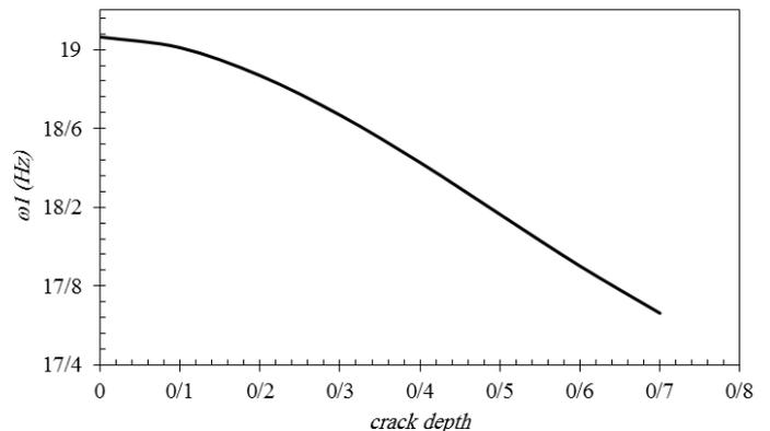
Figure 9. variations of first frequency of plate against crack depth ( $h/a = 0/1$ )
