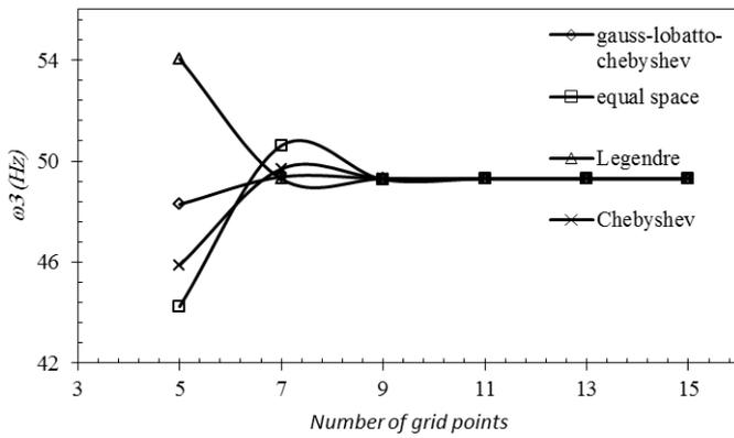
Figure 5. variations of third frequency of plate against the number of nodes
