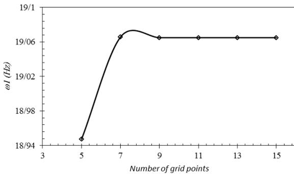
Figure 6. variations of first frequency of plate against the number of nodes
