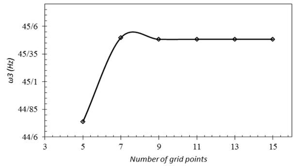
Figure 8. variations of third frequency of plate against the number of nodes
