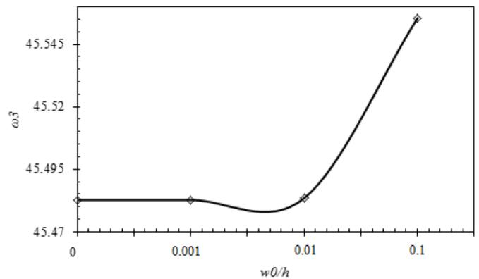
Figure 20. variations of third frequency of plate against initial geometric imperfection amplitude
