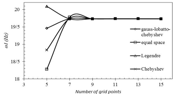
Figure 3. variations of first frequency of plate against the number of nodes
