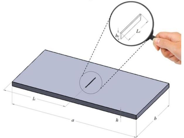
Figure 1. Cracked rectangular plate
