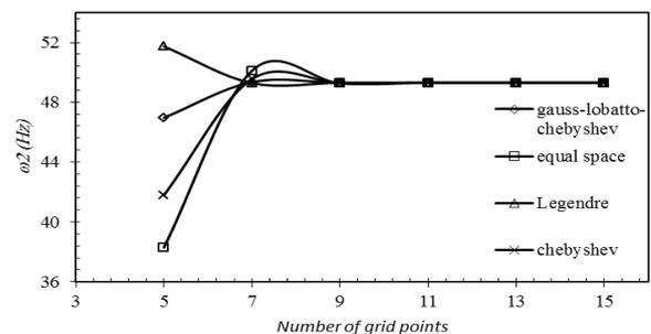
Figure 4. variations of second frequency of plate against the number of nodes
