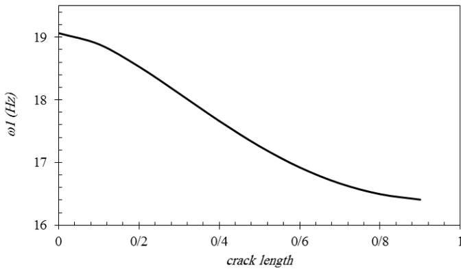
Figure 15. variations of first frequency of plate against crack length ( $h/a = 0/1$ )
