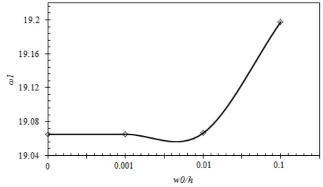
Figure 18. variations of first frequency of plate against initial geometric imperfection amplitude
