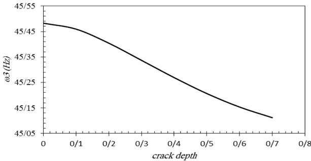
Figure 11. variations of third frequency of plate against crack depth ( $h/a = 0/1$ )
