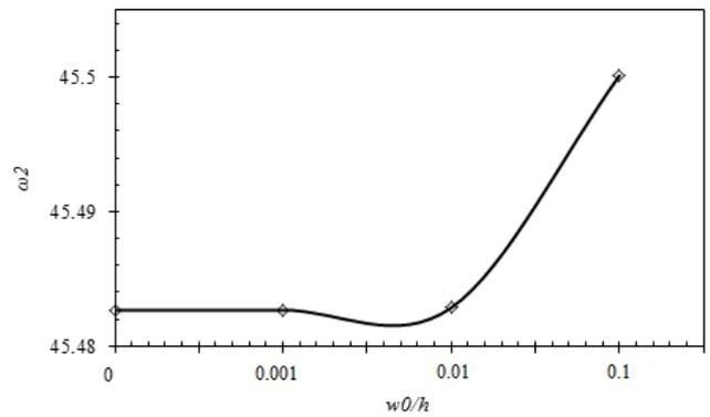
Figure 19. variations of second frequency of plate against initial geometric imperfection amplitude
