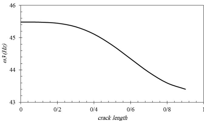
Figure 17. variations of third frequency of plate against crack length ( $h/a = 0/1$ )
