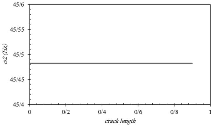
Figure 16. variations of second frequency of plate against crack length ( $h/a = 0/1$ )
