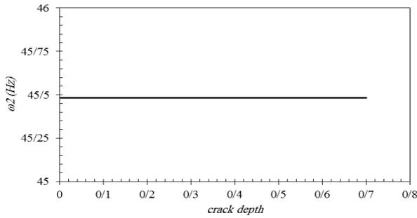
Figure 10. variations of second frequency of plate against crack depth ( $h/a = 0/1$ )
