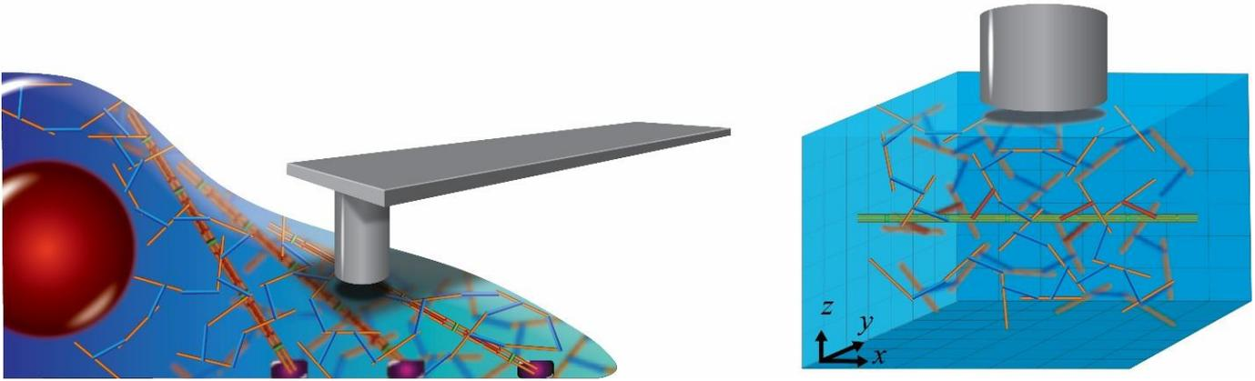
Figure 1. Schematic of an AFM Measuring the Stiffness of Cell Cytoskeleton (Left: The Cell, Right: Simulation Box)
