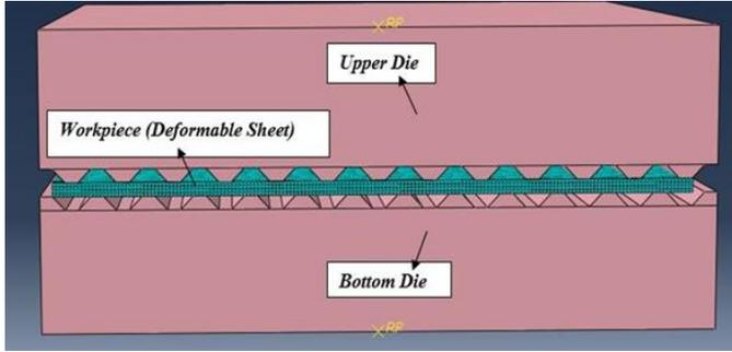
**Figure 2.** Finite element model of constrained groove pressing operation created in ABAQUS.
