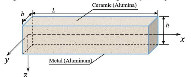
Figure 1: Schematic diagram for the FG nanobeam.
