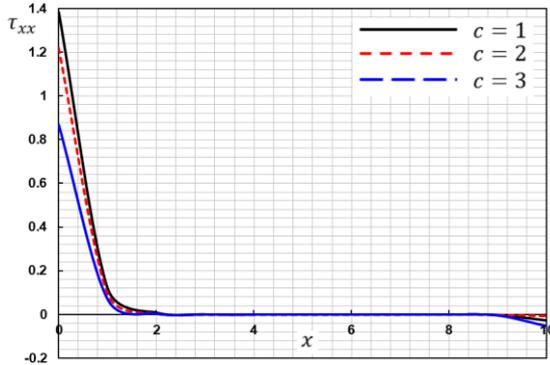
Figure 7: The nonlocal stress  $\tau_{xx}$  with different values of moving heat source velocity  $c$ .
