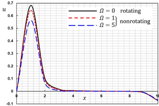
Figure 2: The displacement  $u$  with different rotation parameter  $\Omega$ .
