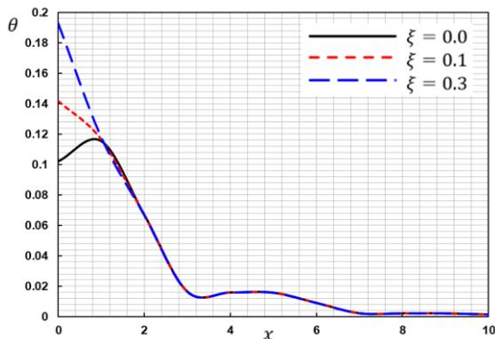
Figure 9: The temperature  $\theta$  with different values of nonlocal parameter  $\xi$ .
