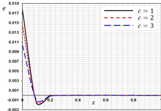
Figure 8: The strain distributions  $e$  with different values of moving heat source velocity  $c$ .
