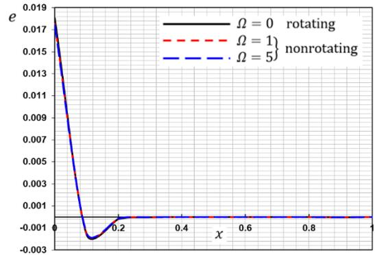
Figure 4: The strain distributions  $e$  with different rotation parameter  $\Omega$ .
