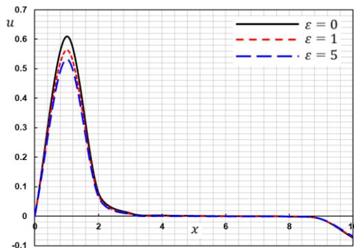
Figure 14: The variation of displacement  $u$  with the applied magnetic field.
