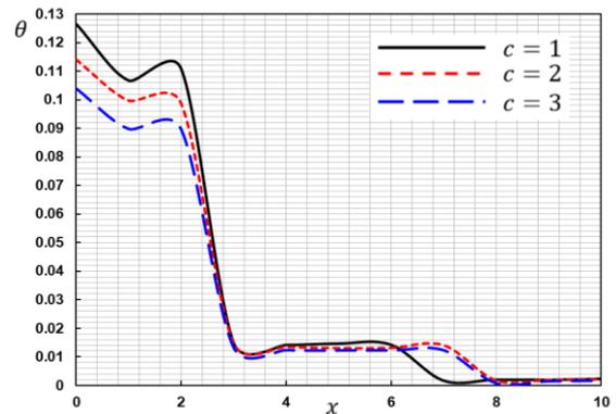
Figure 5: The temperature  $\theta$  with different values of the moving heat source velocity  $c$ .
