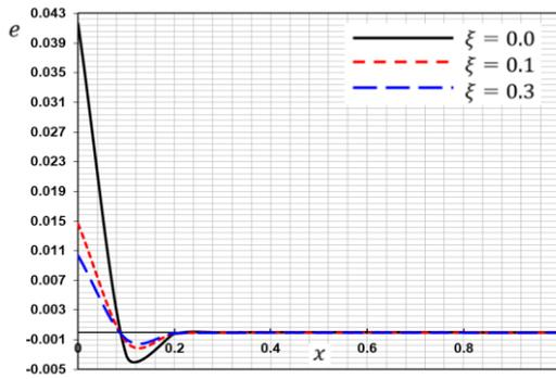
Figure 12: The strain distributions  $e$  with different values of nonlocal parameter  $\xi$ .
