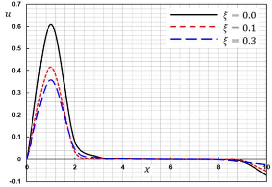
Figure 10: The displacement  $u$  with different values of nonlocal parameter  $\xi$ .
