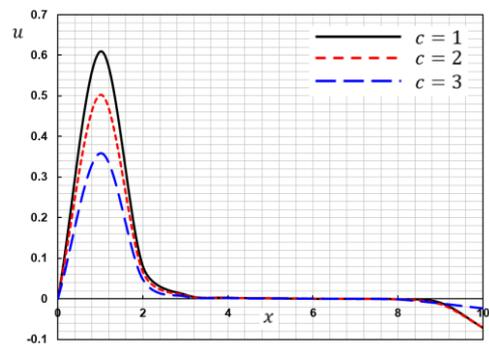
Figure 6: The displacement  $u$  with different values of moving heat source velocity  $c$ .
