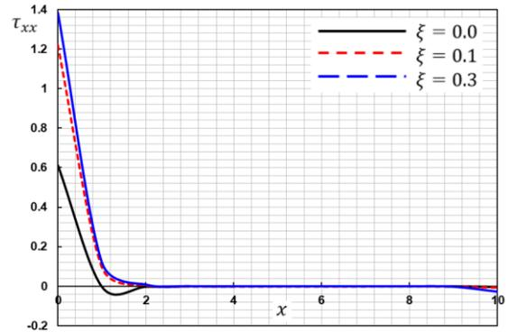
Figure 11: The nonlocal stress  $\tau_{xx}$  with different values of nonlocal parameter  $\xi$ .
