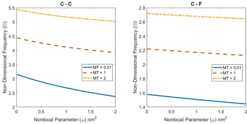
Figure 3. Variation of NDFP with Nonlocal Parameter ( $L=5\text{nm}$ )
