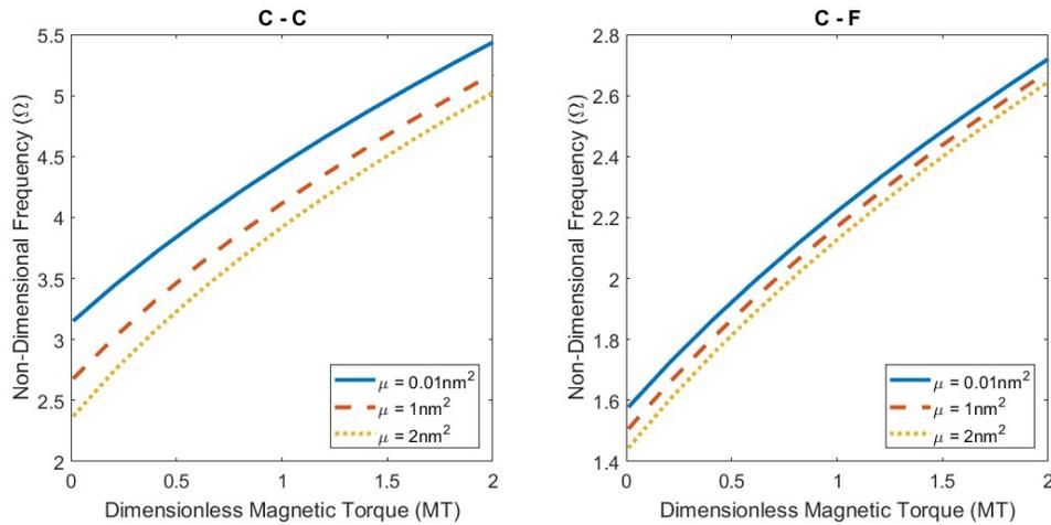
Figure 5. Variation of NDFP with Dimensionless Magnetic Torque (MT) ( $L=5\text{nm}$ )
