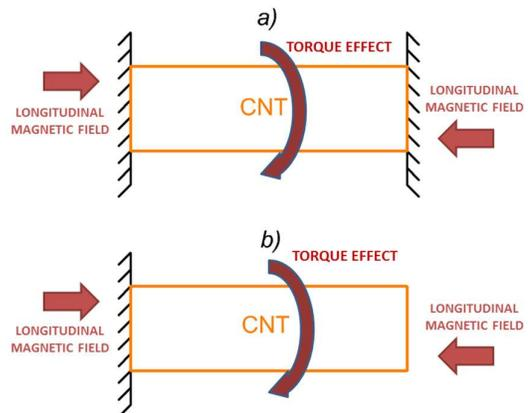
Figure 2. Continuum Model of the Present Problem a) Clamped-Clamped b) Clamped-Free
