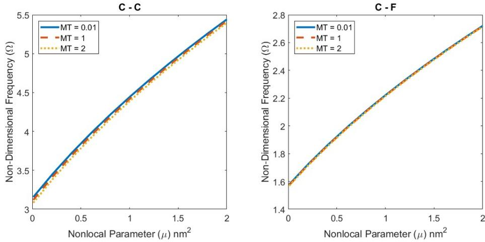
Figure 6. Variation of NDFP with Dimensionless Magnetic Torque (MT) ( $L=20\text{nm}$ )
