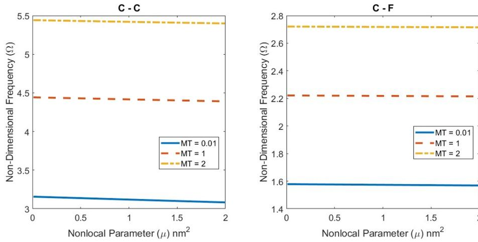
Figure 4. Variation of NDFP with Nonlocal Parameter ( $L=20\text{nm}$ )
