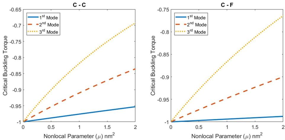
Figure 10. Variation of Critical Buckling Torque with Nonlocal Parameter ( $L=20\text{nm}$ )
