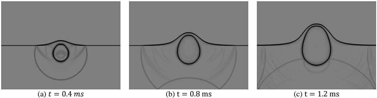
Figure 7. Density schlieren images of numerical simulation of under-water explosion.
