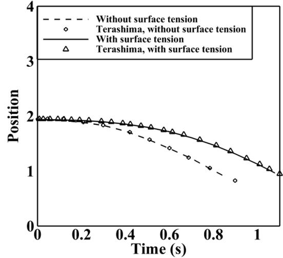
Figure 11. Spike front position in comparison with the results of Terashima, Tryggvason [39].
