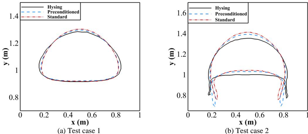
Figure 16. Comparison the simulated bubble shape by preconditioned and standard method with the results of Hysing, Turek, Kuzmin, Parolini, Burman, Ganesan, Tobiska [49] at  $t = 3$  s.
