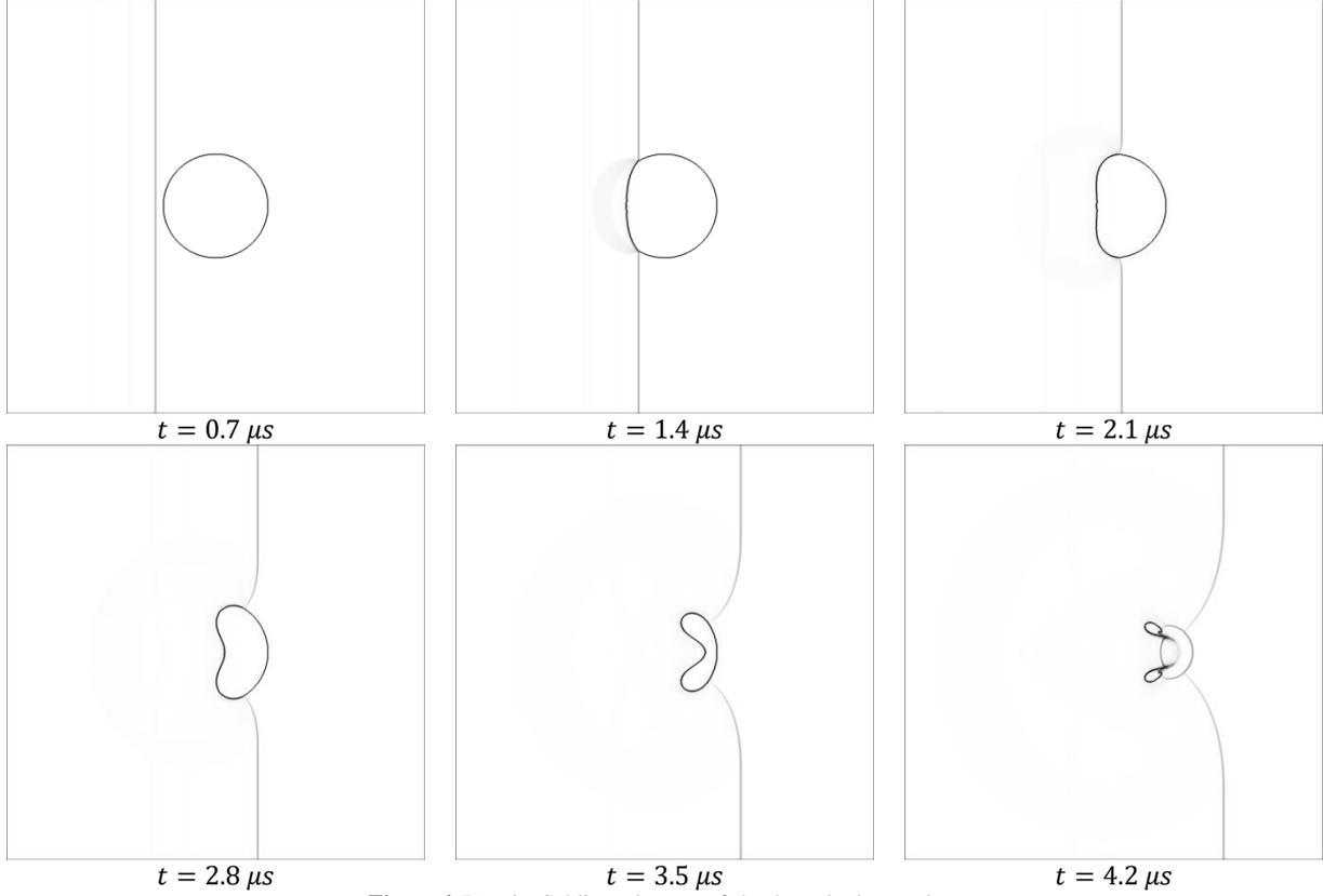
Figure 4. Density Schlieren images of shock-cavity interaction.
