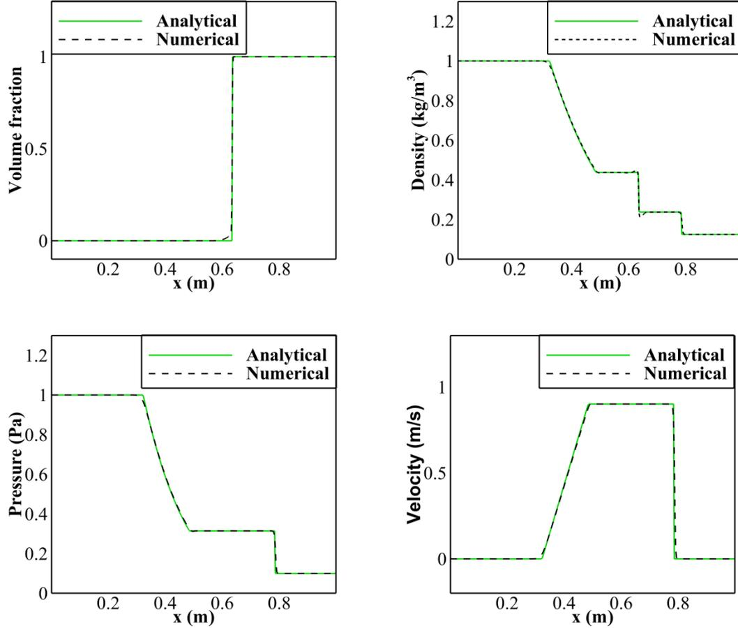
Figure 3. Air-helium shock tube problem at  $t=0.15s$ , solid lines indicate exact solution while dashed lines indicate the numerical solution.
