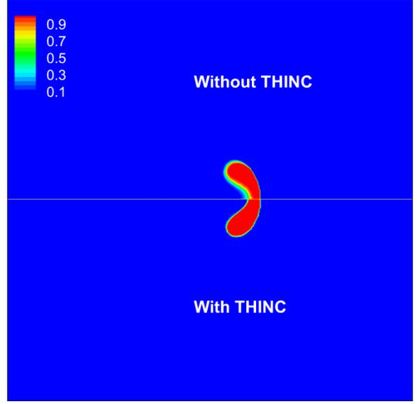
Figure 6. Comparison of interface of shock-cavity interaction at  $t = 3.5 \mu s$ .
