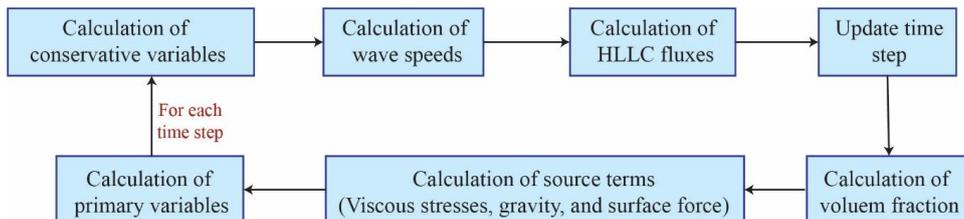
Figure 2. Flowchart of the solution procedure.
