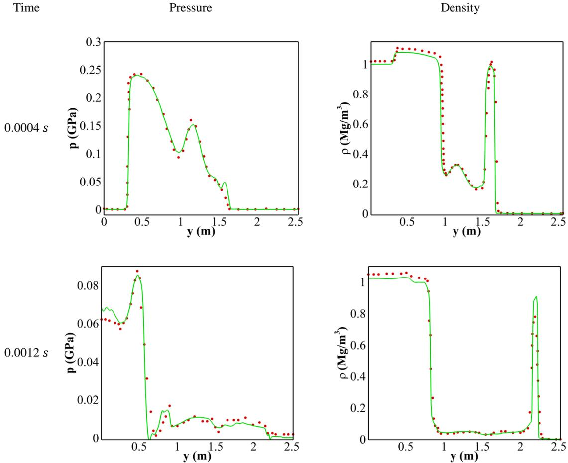
**Figure 8.** Density and pressure distribution of under-water explosion along vertical centerline. Solid lines are the results obtained using the DIM code and the dotted points are the results from Shyue [43] using interface capturing method.
