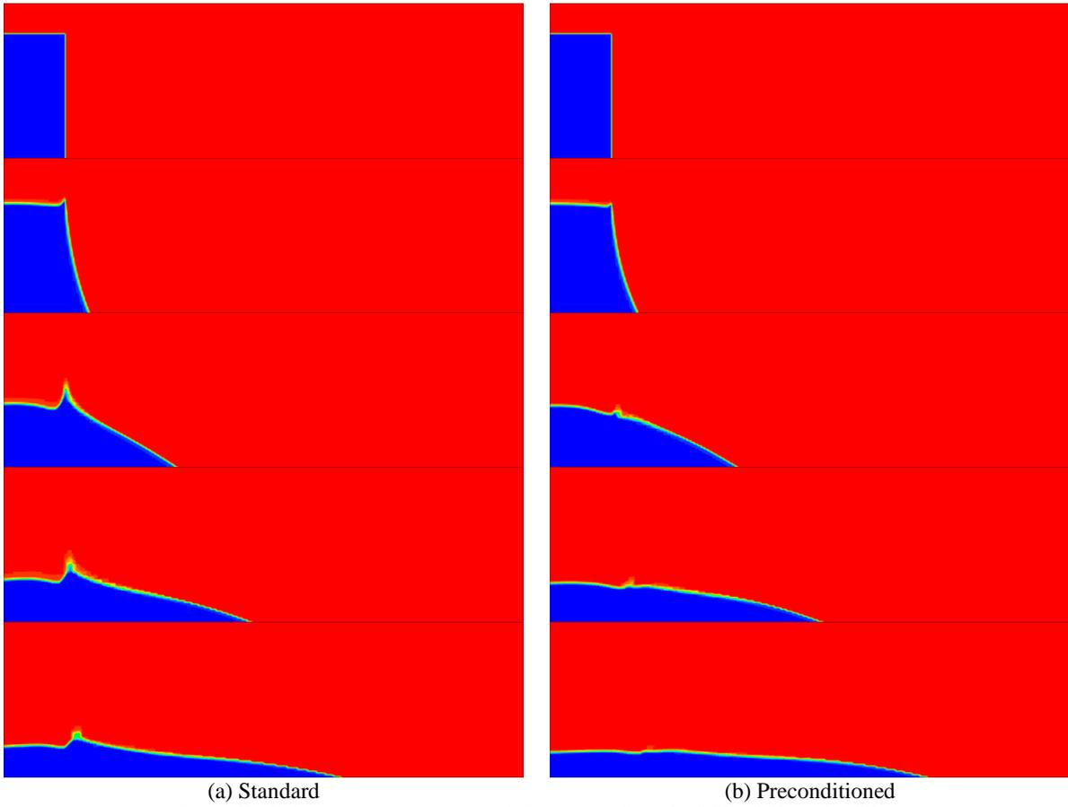
Figure 12. Broken dam simulation at five different times 0, 0.06 s, 0.15 s, 0.21 s and 0.281 s.
