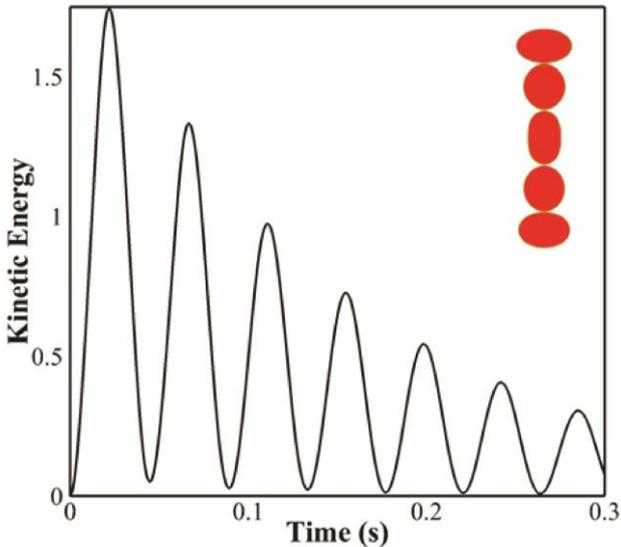
**Figure 9.** Changes of the kinetic energy of an oscillating drop vs. time.
