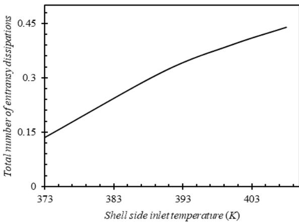
Figure 7. Variations of total entransy dissipation number with the shell side inlet temperature.
