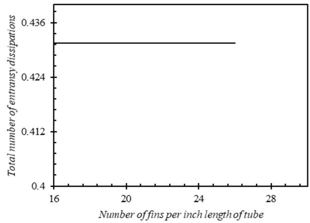
Figure 9. Variations of total entransy dissipation number with the number of fins per inch length of tube.
