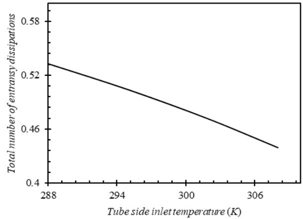
Figure 8. Variations of total entransy dissipation number with the tube side inlet temperature.
