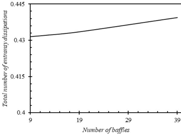
Figure 6. Variations of total entransy dissipation number with the number of baffles.
