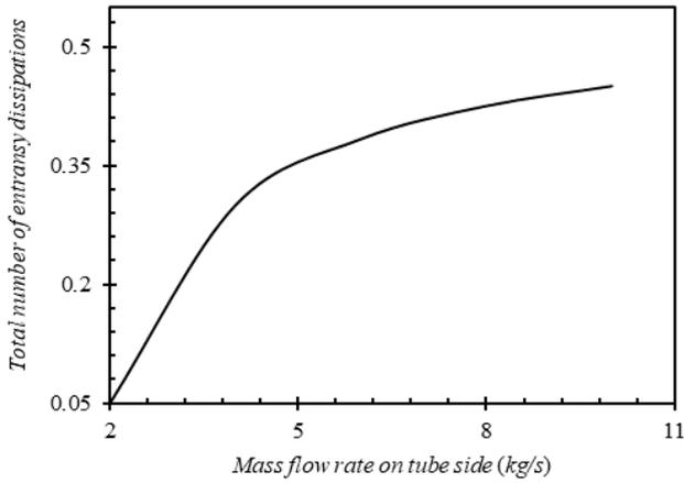
Figure 5. Variations of total entransy dissipation number with fluid mass flow rate
