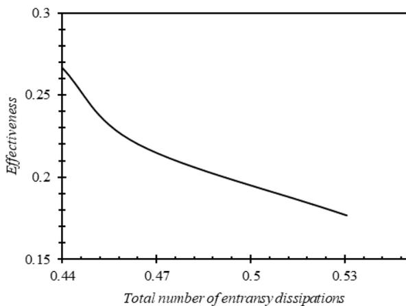
Figure 4. Variation of effectiveness based on the total number of entransy dissipations.
