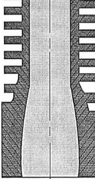
Figure 2. Schematic illustration of a radial low-fin tube [24].
