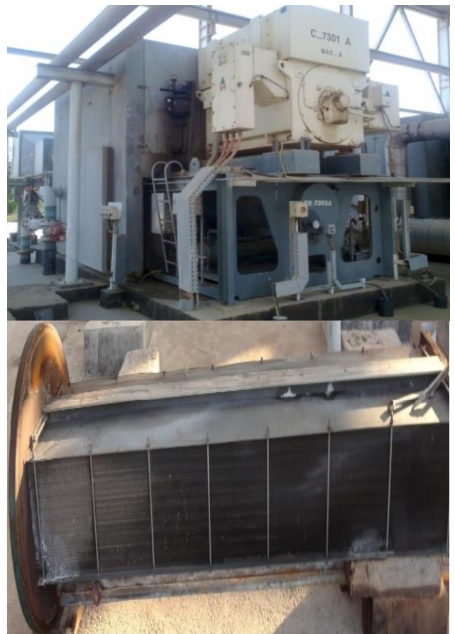
Figure 2. Case study compressor and its intercooler.
