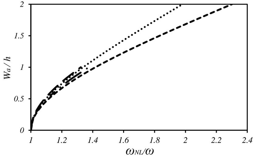
**Figure 2:** Variation of maximum amplitude versus the frequency ratio for different aspect ratio. ( $a/b=1$  (...),  $a/b=2$  (---),  $a/b=1$  Mei [2] (-.),  $a/b=2$  Mei[2] (-.-))
