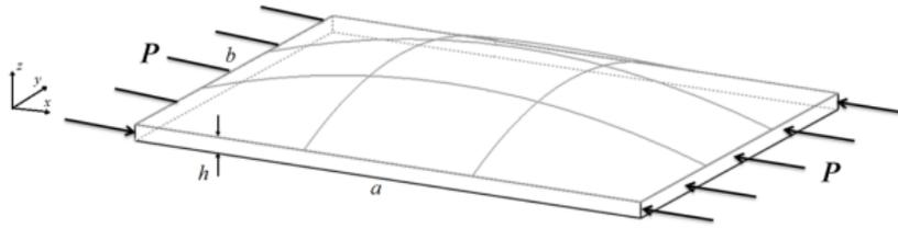
**Figure 1.** A rectangular plate with initial imperfection under uniaxial compressive load.
