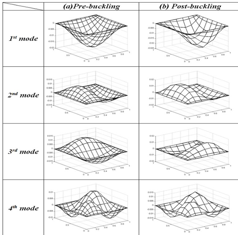
**Figure 4:** Nonlinear modal shapes of the simply supported plate: (a) Pre-buckling (b) Post-buckling.
