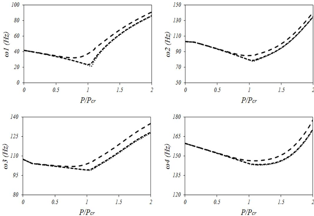
**Figure 5:** variation of the first four nonlinear frequencies of a simply supported square plate with applied load for different initial imperfection. ( $W_0/h=0.001$  (...),  $W_0/h=0.01$  (---),  $W_0/h=0.1$  (—))
