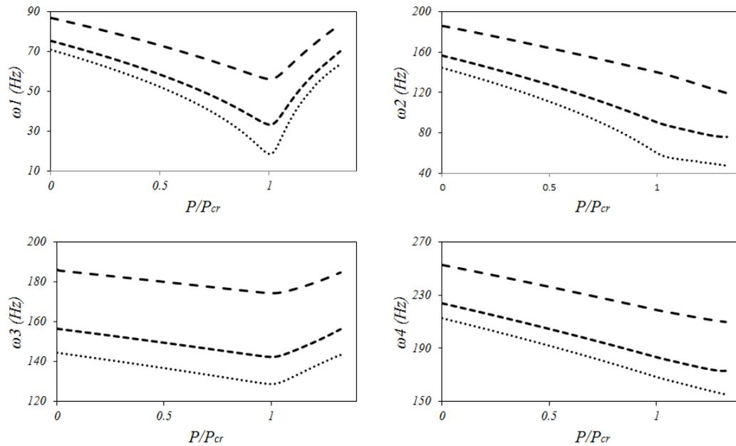
**Figure 7:** variation of the first four nonlinear frequencies of a fully clamped square plate with the compressive load for different amplitude. (linear (...),  $W_a/h=0.5$  (---),  $W_a/h=1$  (-))
