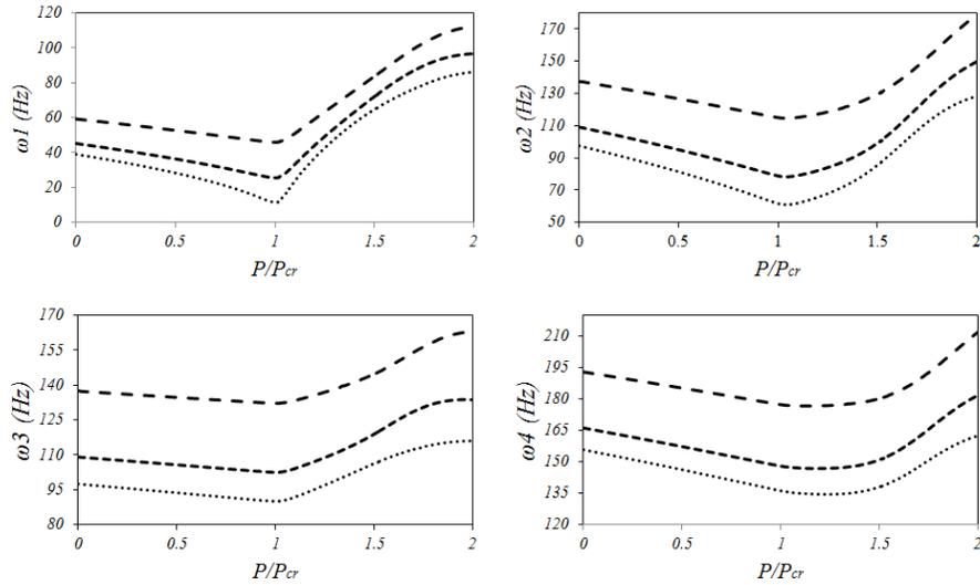
**Figure 3:** variation of first four natural frequencies of a plate against compressive load for different vibration amplitude.
