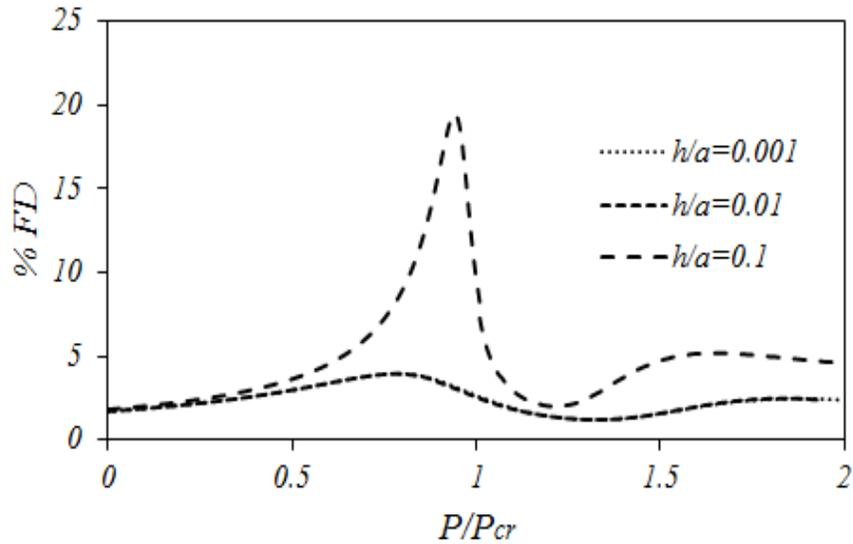
**Figure 6:** Effect of plate thickness on first nonlinear frequency. ( $h/a=0.001$  (...),  $h/a=0.01$  (---),  $h/a=0.1$  (-))
