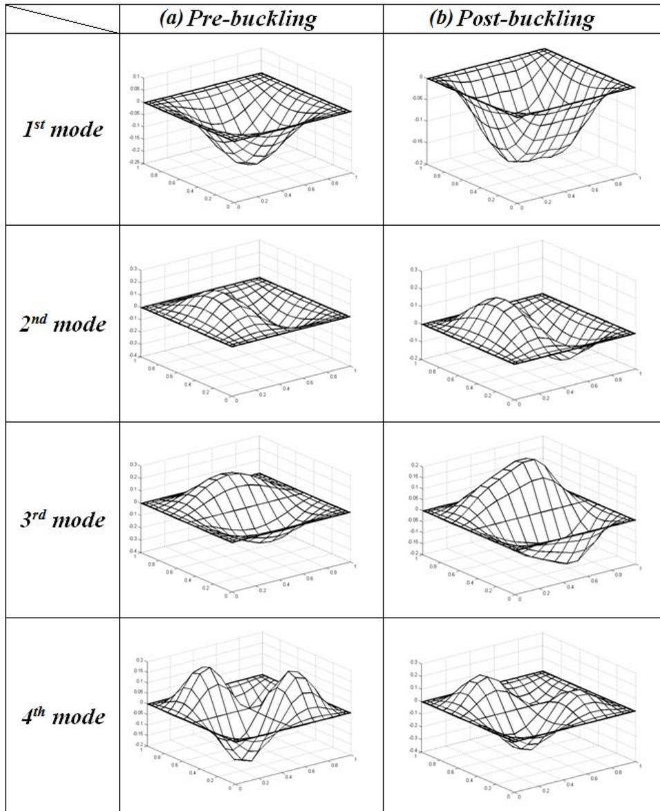
**Figure 8:** nonlinear modal shapes of the fully clamped plate: (a) Pre-buckling (b) Post-buckling.
