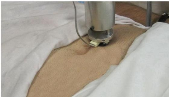
Figure 11. Human's abdomen under indentation test using prototype device
