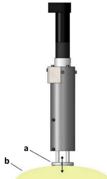
Figure 1. Basic design of tactile device: (a) sensor plate; (b) abdomen
