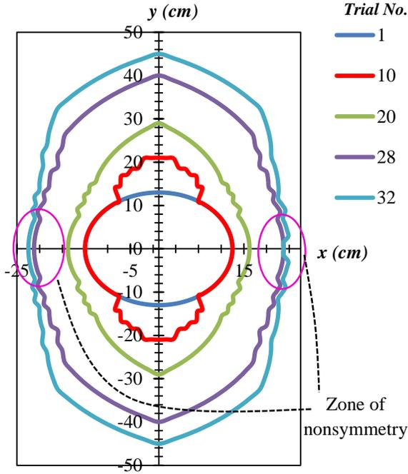
Fig. 16. Delamination growth process in [90//0/0/90/90/0/0/90] sample.
