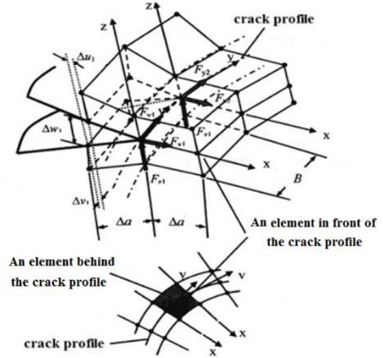
Fig. 1. Elements surrounding a three-dimensional crack tip.
