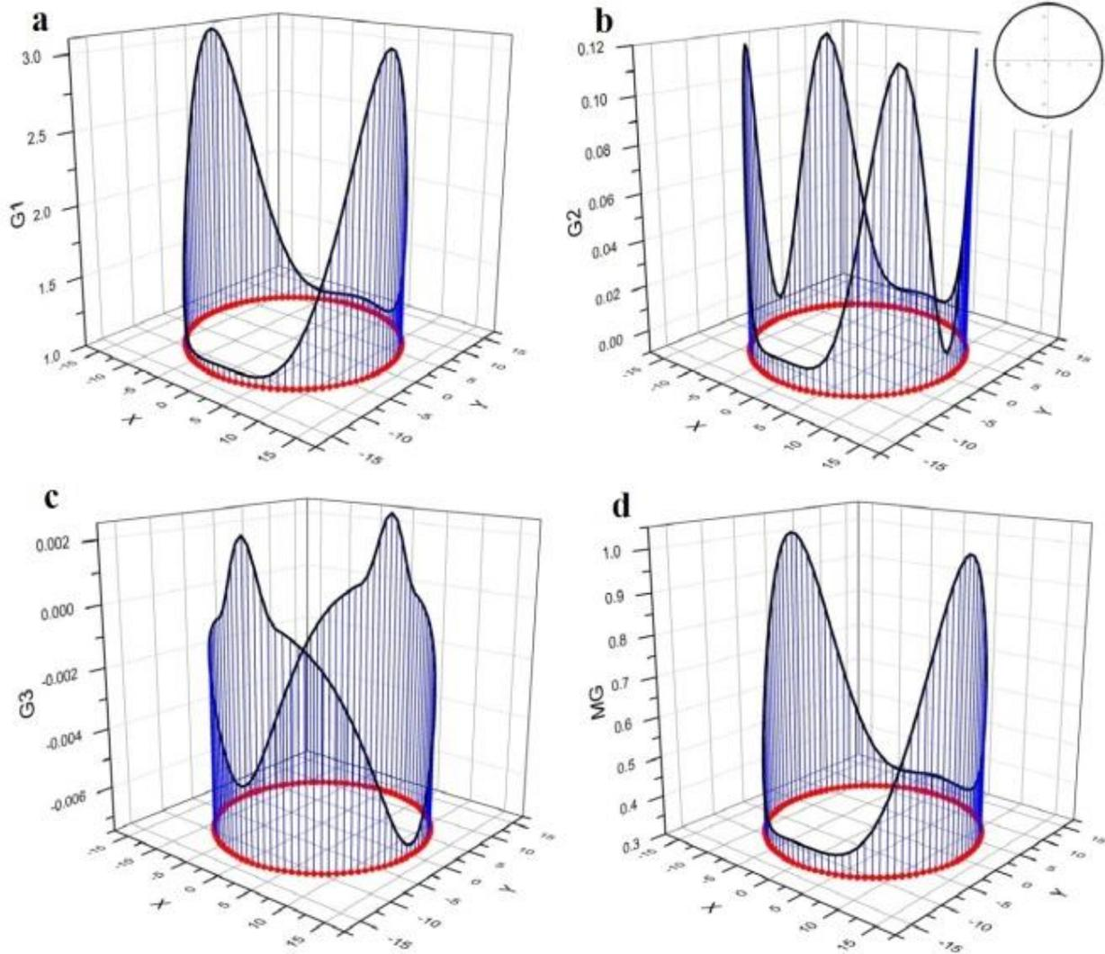
Fig. 8. Strain energy release rate curves for  $[0/90/90/0/0/90/90/0]$  sample: a- Strain energy release rate of the first mode, b- Strain energy release rate of the second mode, c- Strain energy release rate of the third mode, d- growth criteria.
