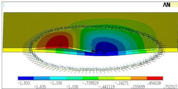
Fig. 11. Buckling mode at the latest stage of delamination growth (fortieth step) in [0/90/90/0/0/90/90/0] sample.
