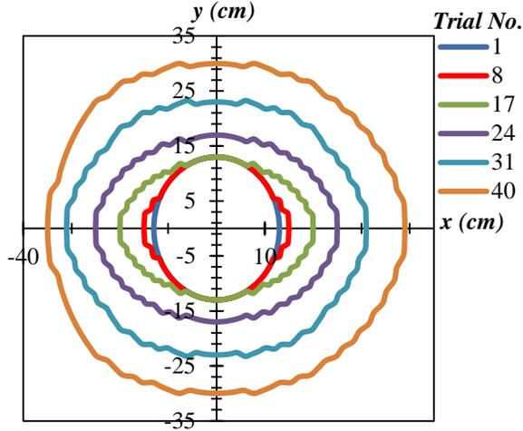
Fig. 10. The delamination growth process in [0/90/90/0/0/90/90/0] sample.
