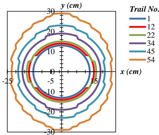
Fig. 5. The delamination growth process in [0/90/90/0/0/90/90/0] sample.
