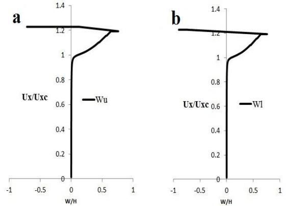
Fig. 13. Out-of-plane displacement of the node located at the center of the plate for [0/90/90/0/0/90/90/0] sample: a- Displacement of the node located at the top of the delaminated region, b- Displacement of the node located at the bottom of the delaminated region.
