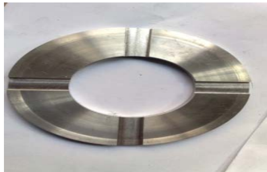
Figure 5- Final disk that was product with machining
