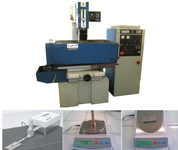
Fig. 2. Die-sinking EDM machine, Digital surface roughness tester and electronic balance used
