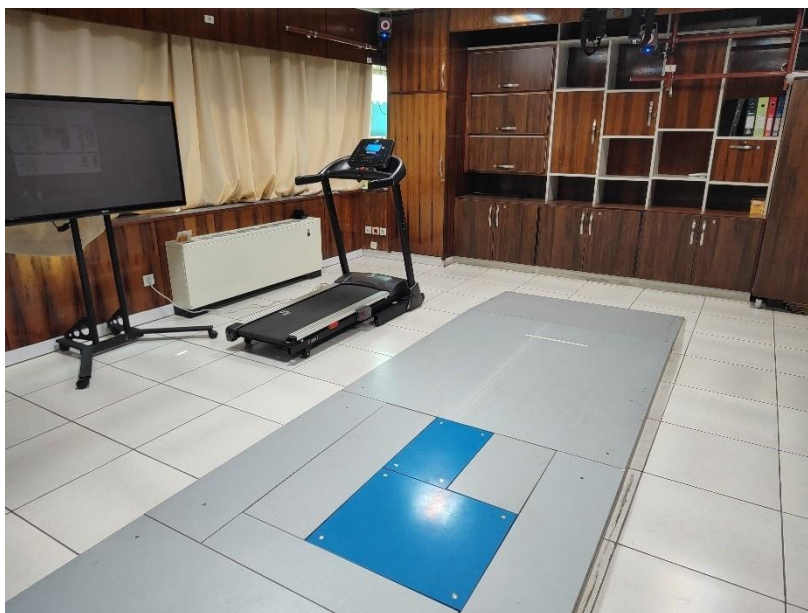
Fig 4: An image of the walking path, the location of the force plates (blue-colored plates), and the treadmill
